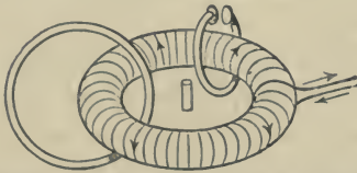
FIG. 47.—Closed magnetic circuit like Fig. 42, with a single-ring secondary circuit, and another open secondary loop ; also with a short conducting-rod standing in it.
